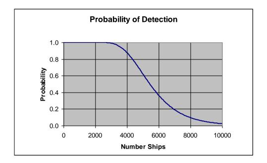
Figure 1. Probability of Detection of Class A Message in Class B environment.
